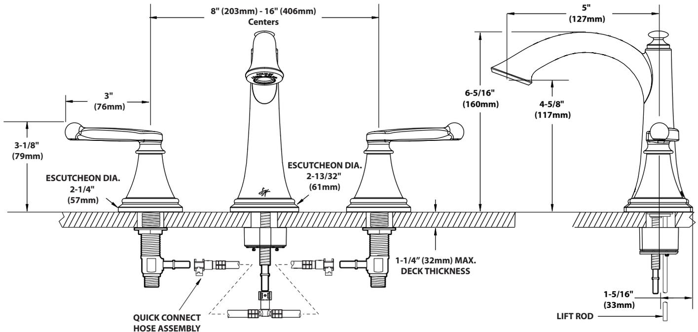
**NOTE:** FOR DECK THICKNESS 1-3/8" - 3", USE SERVICE KIT #115001. VALVES INSTALL THROUGH 1-1/4" DIA. HOLE
