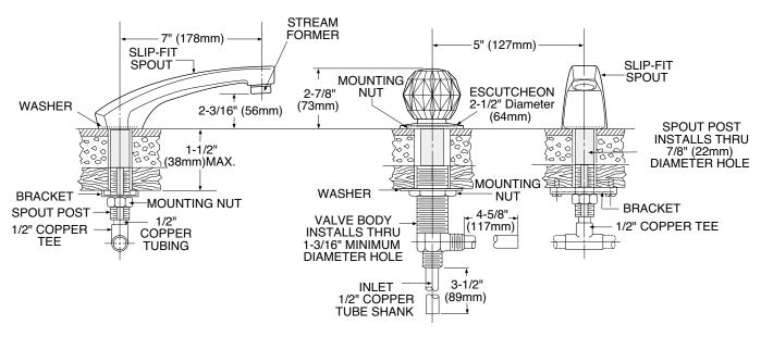
NOTE: THE INSTALLATION SHOWN IS FOR TILE DECKS, THIS VALVE WILL ALSO FIT STEEL, CAST IRON OR PLASTIC DECKS
