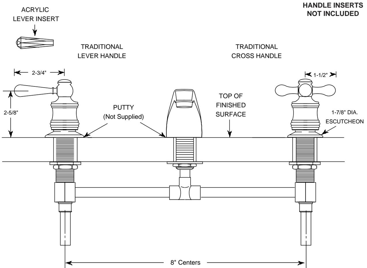
**CAUTION:** Always turn water OFF before disassembling faucet. Open faucet handles to relieve water pressure and to insure that COMPLETE water shut-off has been accomplished.
