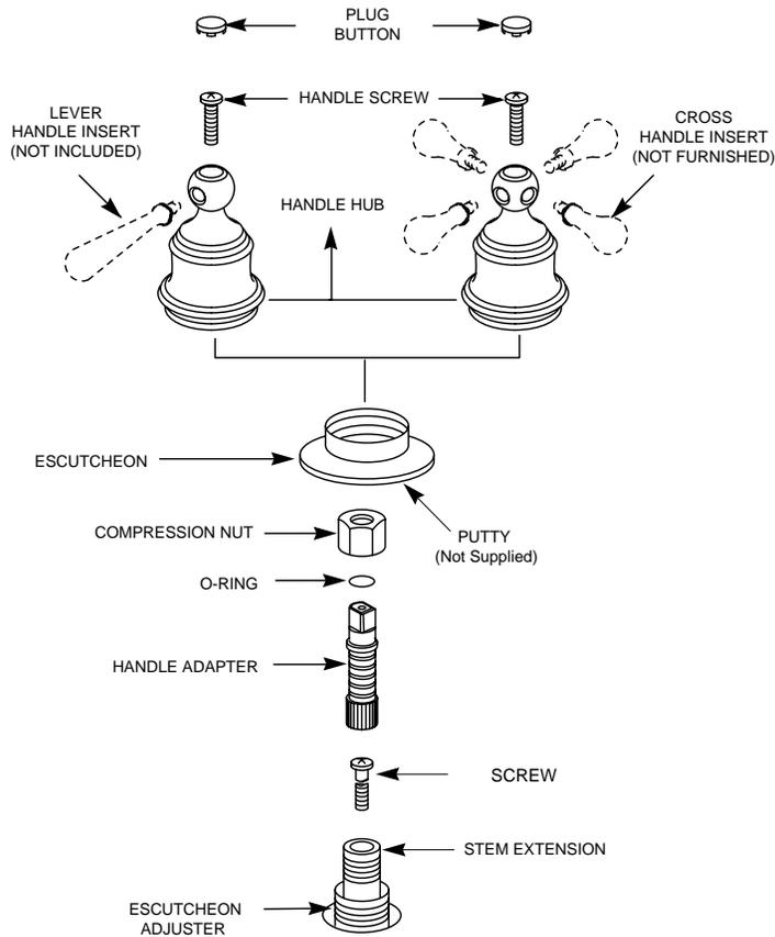
1. Apply a 3/8" of plumbers putty (not furnished) around mounting nut on finished tub base.
