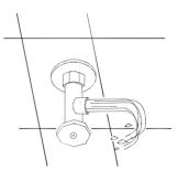
1. Flush water supply lines to remove any debris that has accumulated in the supply lines that could damage the faucet.
