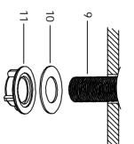
3. From below, assemble the lower deck gasket (10) and mounting nut(11) to the mounting stud(9). Tighten the mounting nut (do not overtighten). Connect the inlet supply line (purchased separately) to the mounting stud and the water supply line.
