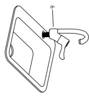
2.Be sure the mounting surface is dry and clean. Guide the mounting stud of the valve body(6) through the deck. Position the faucet on the mounting deck.
