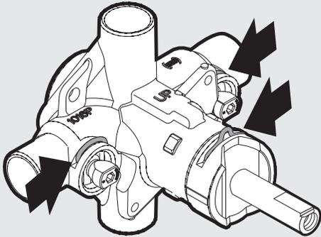
Ensure retainer clips are installed prior to escutcheon installation.
