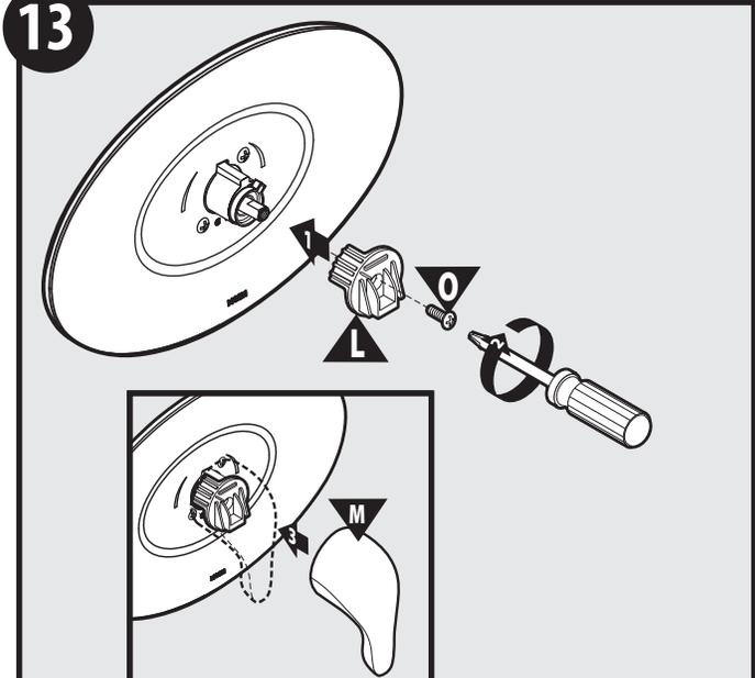
Remove the lever (M) and lever handle adapter (L). Note the position of the stop. Position the adjustable temperature limit stop (D) so the lever stops at that position. This prevents the lever from being turned into an unsafe temperature. After setting the adjustable temperature limit stop to the desired position, reattach the lever handle adapter (L), adapter screw (O), and lever (M). Make sure ridges on back of (L) are to the left of the tab on (D).
