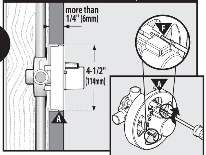
The "Thin Wall" method is used when the tub/shower wall is less than 1/4 inches thick (such as fiberglass tub surround) and will be the main source of support for the valve. The plaster ground (A) remains attached to the valve. A 2-1/4 inches to 3-1/2 inches diameter hole is cut thru the wall for this method. Break away the black plastic protective cover using pliers and rotating clockwise.
